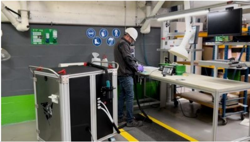
Thanks to the system's cutting-edge technique of non-drip selective plating, all chemical solutions flow and vacuum through the SMART tools before being recycled back into the cart's solution management system - right at the surface of the workpiece. The result is a cleaner, more environmentally friendly, and inherently safer working environment.
